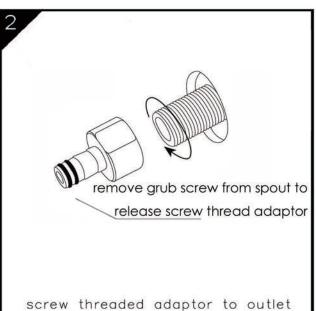
tighten firmly with allen key
